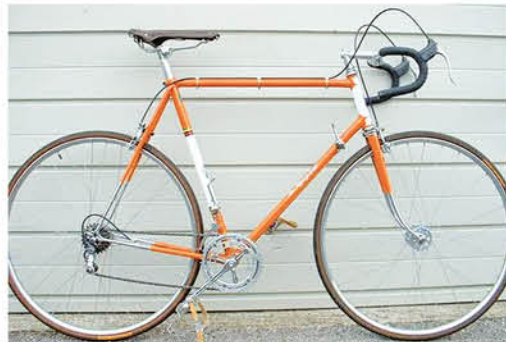
1953 'Flying Scot' Continental Supreme, built with Reynolds 531 tubing and Nervex Professional Lugs.
